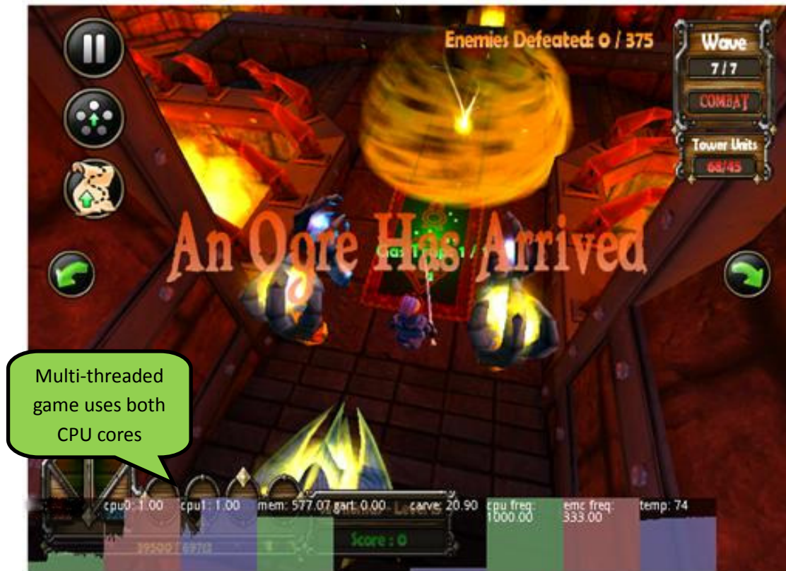
Figure 9 - Dungeon Defender using both cores of the NVIDIA Tegra Processor
